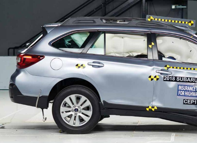
Front passenger protection in small overlap crashes is the focus of a new IIHS test program. Most midsize cars performed well, but airbag protection was inconsistent.
