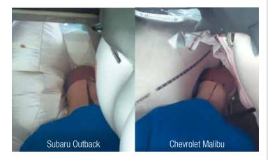
In the passenger-side small overlap test of the Subaru Outback (left), the passenger dummy's head hit the front airbag and stayed there until rebound. In the Chevrolet Malibu's test (right), the passenger dummy's head went between the front and side curtain airbags and hit the dashboard.
