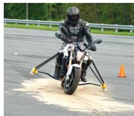
A rider demonstrates a motorcycle equipped with ABS on the Institute’s test track.
