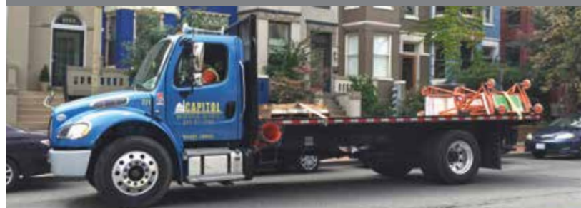
Single-unit trucks like these are exempt from National Highway Traffic Safety Administration requirements for rear underride guards. The agency is considering closing that loophole. Underride guards prevent smaller vehicles from going underneath a truck in a crash.
