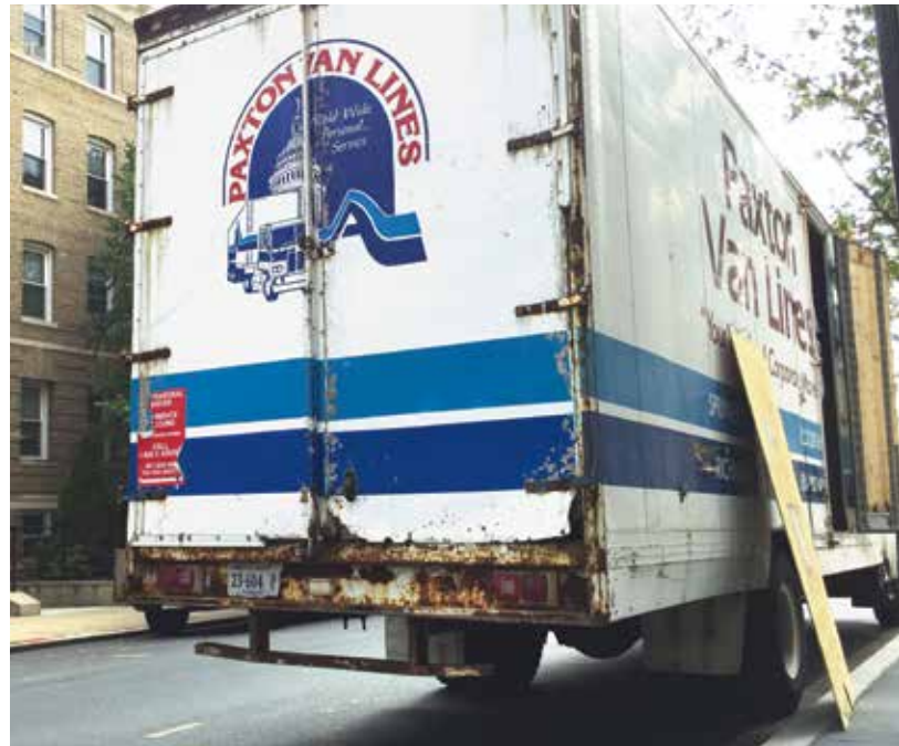
Single-unit trucks like these are exempt from National Highway Traffic Safety Administration requirements for rear underride guards. The agency is considering closing that loophole. Underride guards prevent smaller vehicles from going underneath a truck in a crash.
