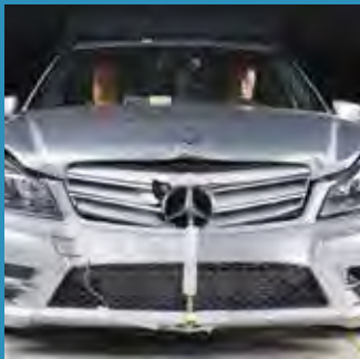
12 mph test: Mercedes-Benz C-Class into rear of Chevrolet Malibu
