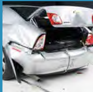
12 mph test: Mercedes-Benz C-Class into rear of Chevrolet Malibu
