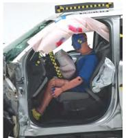
man was positioned at the steering wheel. The test replicates what happens when the front corner of a vehicle collides with another vehicle or an object such as a tree or a utility pole.
