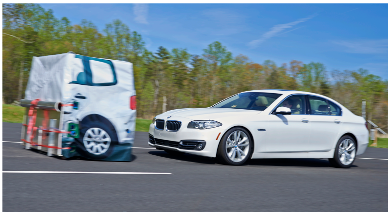
The BMW 5 series brakes for the target in an IIHS test. The car earns a superior rating when equipped with an optional camera and radar system.
