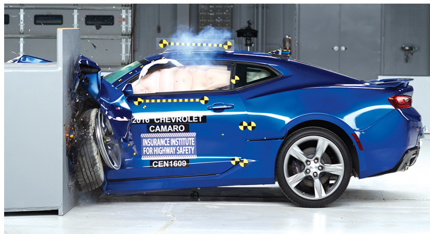
The 2016 Chevrolet Camaro earns a good rating for occupant protection in a small overlap front crash. The Camaro's safety cage resisted intrusion.
