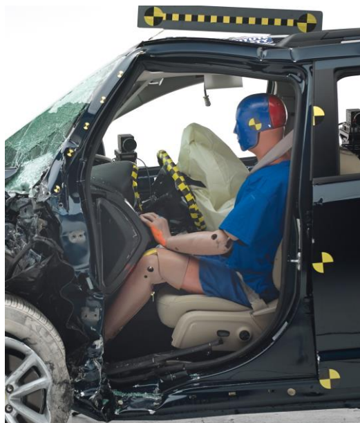
BEST AND WORST: The Nissan Murano's structure (top) held up well. In contrast, the occupant compartment of the Dodge Journey (bottom) collapsed.
