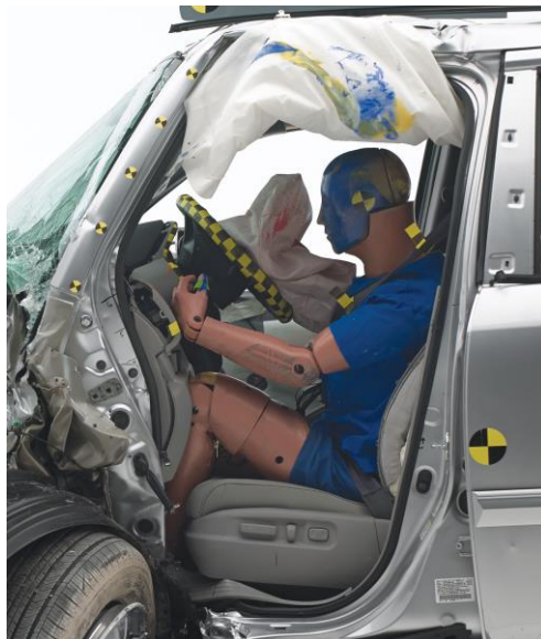
The structure of the Chevrolet Equinox (top) held up well, while the driver's space was badly compromised in the Honda Pilot.
