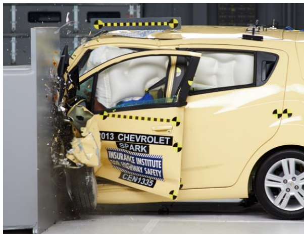
The Chevrolet Spark is the only minicar tested to earn an acceptable rating in the small overlap front test.
